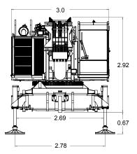
Superstructure Transport Weight:29,015 kg (Standard crane with 4 section 34 m boom, Aux winch with wire rope, carbody jacks)
